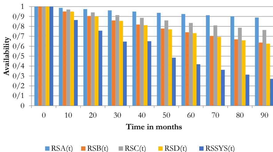
**Fig. 2. Availability comparison between subsystems and the entire system.**
